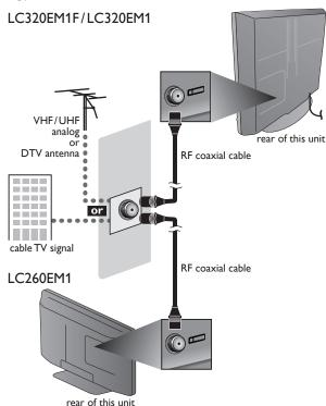
Once connections are completed, turn on the unit and begin initial setup. Channel scanning is necessary for the unit to memorize all available channels in your area. [Initial Setup] • p.15
