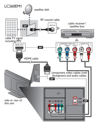
You can also connect this unit to the cable receiver or satellite box other than the HDMI or the component video output jacks because they might have different output jacks.
