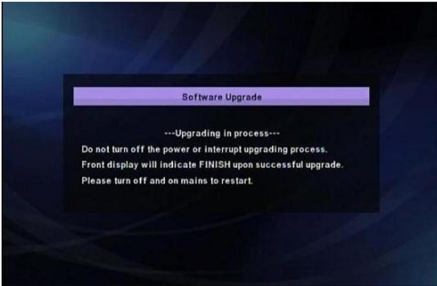
10. After a brief delay, the LED Display on the unit will read “FINISH or GOODBYE” indicating the firmware update completed successfully. At this point, the unit will reboot itself.
