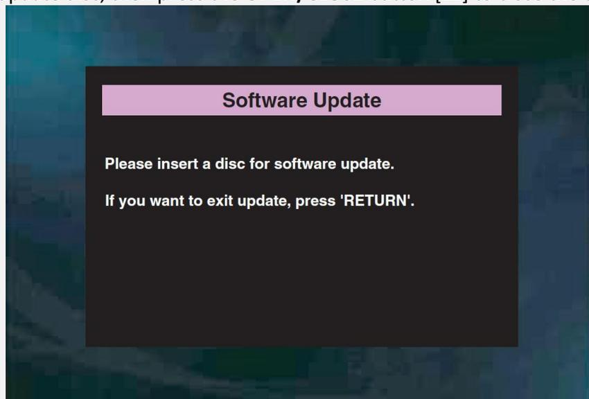
9. The update disc will begin loading automatically. During this process, the front panel display will show **LOADING** and the following screen will appear:
