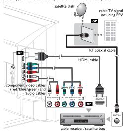
Required cables and connecting methods of the cable receiver/ satellite box, or the availability channel for the clear QAM may differ depending on the cable/satellite provider or local TV broadcaster.
